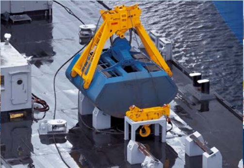
The barge has special mounts on which the hook rotator and grabs of various types and sizes can be set down
