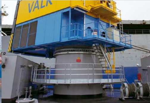
The slew ring of the crane is mounted on a cylindrical pedestal integrated in the barge
